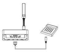
Connect the amplifier: connect XLRM outlet to other equipment, such as microphone amplifier, mixer, etc.
