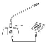
Connect the amplifier: connect XLRM outlet to other equipment ,such as microphone amplifier, mixer etc.
