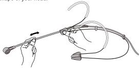
For placement discreetly, you can bend the microphone boom slightly so that the capsule is placed in the desired position. Do not hold the capsule while bending, bend the wire boom, making a smooth curve with your thumb to best fit the profile of the face.
