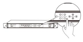
Press MENU to enter the function main menu. (Frequency setting, video tracking setting, mixing setting, system setting)
