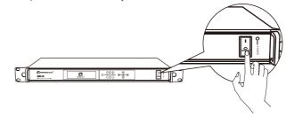
After the system is started, the AMC-20 screen will show the main interface of the system, and observe whether the screen is connected to WAM-432.
