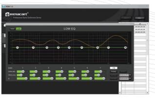
Both the tweeter and woofer can be set with 7-band equalization, high-pass filter and low-pass filter independently
