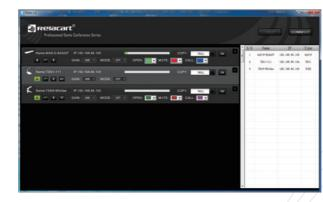
Remotely control microphone mute, gain, low-cut switch, and work mode(ON/OFF/PTM/PTT). The parameters of the same model microphone in the same LAN can be copied with one click
