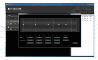
Some microphones support equalization adjustment function, 4-band equalization and high-pass filter can be set by software
