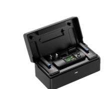
• The charging case can charge the whole kit up to 4 times. It takes only 1.5h to recharge RX and TXs. After fully charged, TX and RX can be used up to 5 hours. If you use two TXs at a time, the whole system can work for 25 hours with the charging case. When taken out of the case, they are automatically turned on. When put inside, they are automatically paired and will start to charge if needed. Ready to use at anytime, anywhere.
