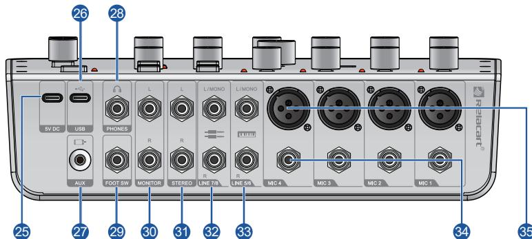
25 5V DC port: used to connect to commercially available USB power adapters or USB mobile power supplies. This port can be used when the mixer is connected to a tablet computer or other device that cannot power the mixer.
