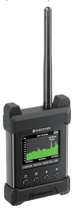
U.Discover is a portable handheld spectrum management controller that adopts an ultra-wideband solution and can scanfrequencies from 240MHz-960MHz. it is equipped with a HD screen to display frequency details, making it clear at a glance the on-site interference frequencies. t can create a stable wireless working environment for the site, making the site frequency visible and controllable.
